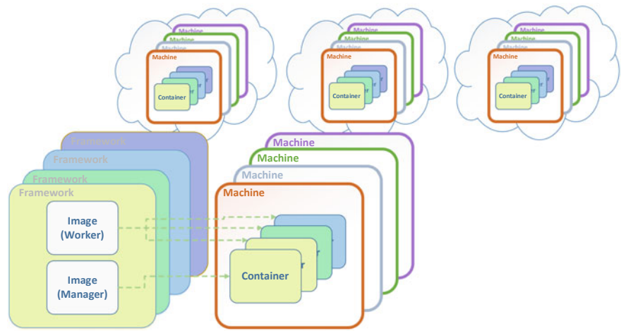
Fig. 3.12 Multi-tenant multi-cloud infrastructure enabled by container technology
