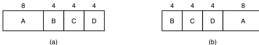
Figure 2-41. An example of shortest-job-first scheduling. (a) Running four jobs in the original order. (b) Running them in shortest job first order.
