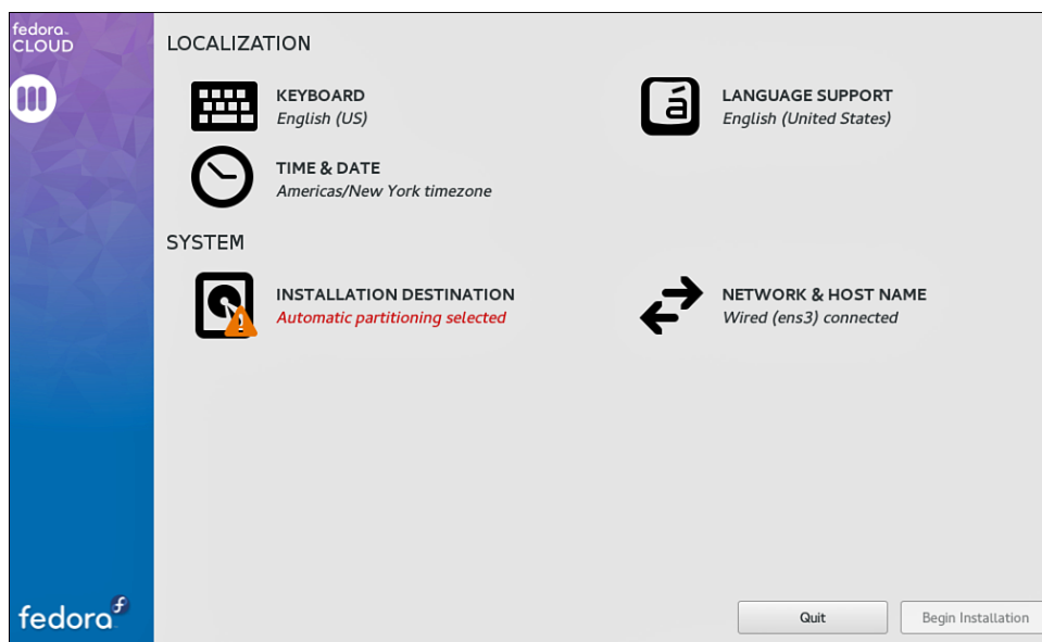
FIGURE 2.1 Identify disk partitions and networking settings from the Installation Summary screen.
