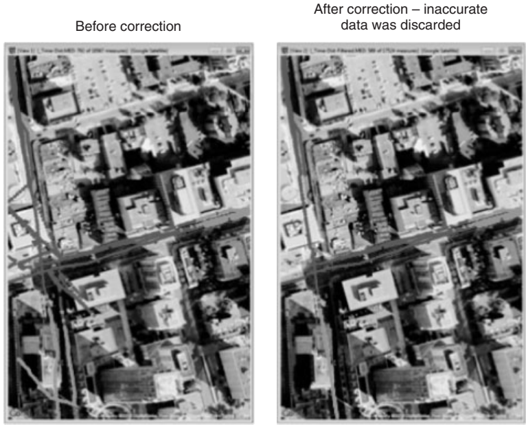
Figure 19.9 GPS errors due to high rise buildings, before and after filtering.
