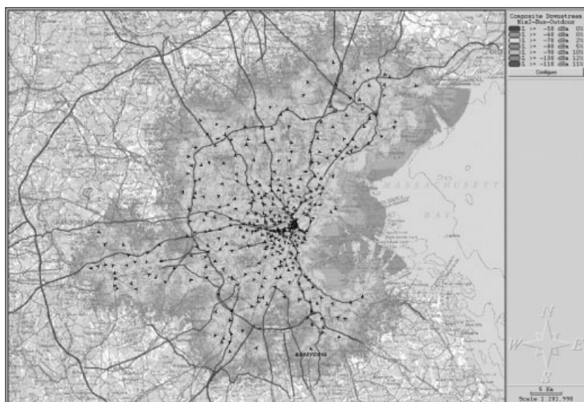
Figure 21.22 Composite signal level downstream at 4th floor.
