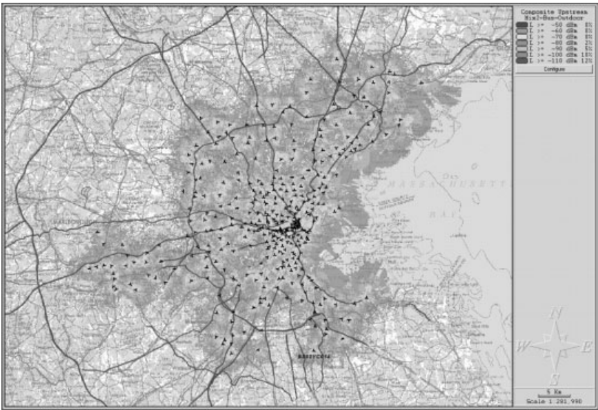
Figure 21.23 Composite signal level upstream at 4th floor.
