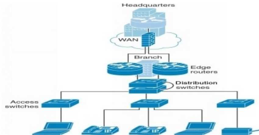
Figure 10: Typical Branch Network Design of Enterprise IPv6
