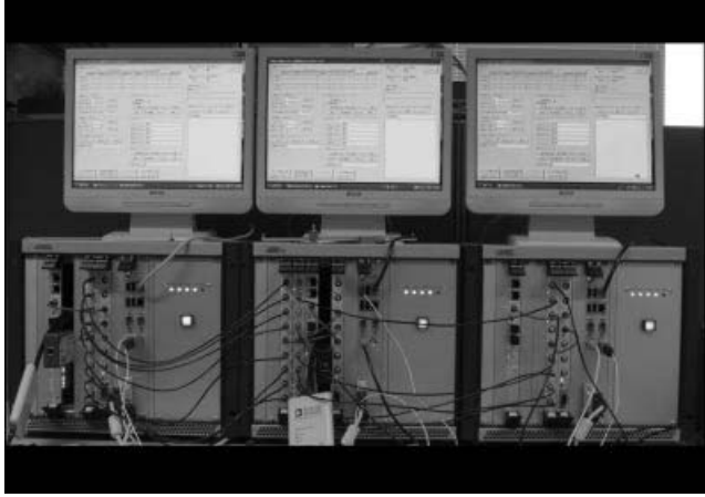
Figure 14.12 Testbed set-up consisting of transmitter, channel emulator and receiver systems.
