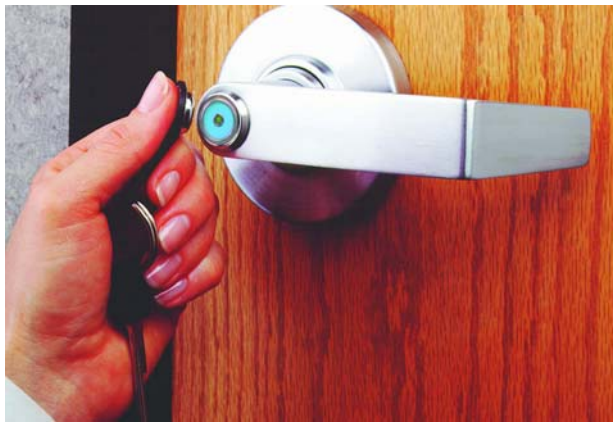
Figure 3.6 Using an iButton to unlock a door by placing the token against a sensor
