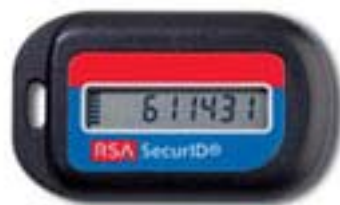
Figure 9.5 The RSA SecurID device that generates a one-time use password
