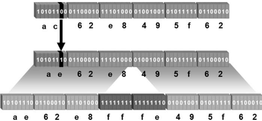
Figure 2-15. Modified EUI-64 interface ID example [28].
