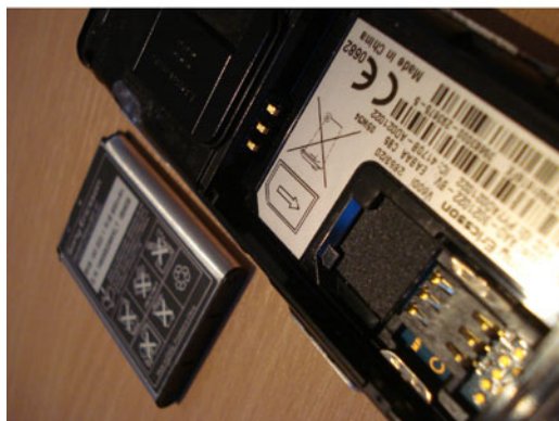
(c) ... which when opened, exposes the power and SIM card interfaces.
